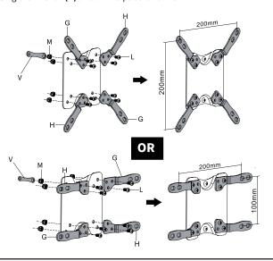
Use bolts (M-A-M-D) along with washers (M-E, M-F) to secure VESA plate with the adapters to the back of your television. Make sure the "VIVO" logo on the front is right side up. For a curved television, spacers (M-G) may be required.
